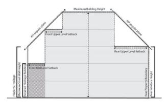
Figure 5. Building envelope requirement – Heritage Building (Figure 1 in Schedule 15 to Clause 43.02 Design and Development Overlay).
