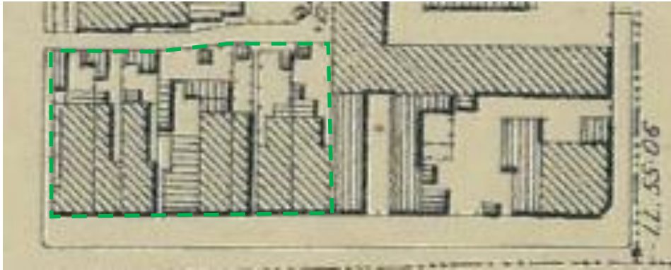
Figure 1. The commercial strip in 1897. The extent of the precinct is indicated in green. Diagonal hatching indicates a brick or stone building, while the horizontal hatching indicates a building constructed of wood (MMBW No 28, dated 1897)
