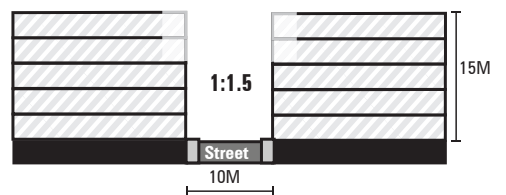
A default street width to building height ratio 1:1.5 for local streets (10-20m) for moderate sized lots
