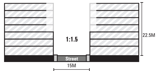
A default street width to building height ratio 1:1.5 for moderate sized lots on Smith and Reeves Streets (20m wide)
