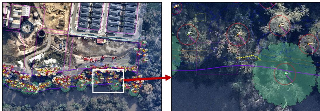
Figures 1&2. Approximate length of soil cracking (yellow dashed line) relative to the closest of the assessed trees. Red circles indicate SRZs.
