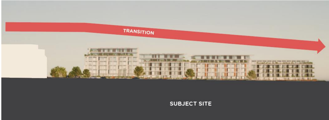
Figure 1 – Built form transition from north to south along Chandler Highway with a reduction in height of one level to both Building A and Building B (Source: Elenberg Fraser with annotations)
