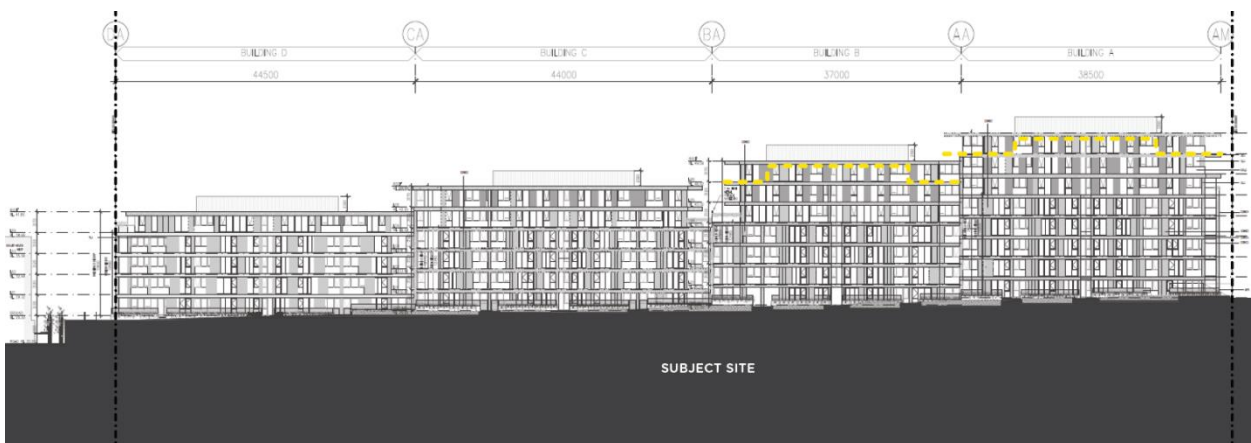
Figure 3 – East elevation showing one level removed from both Building A and Building B (Source: Elenberg Fraser with annotations)
