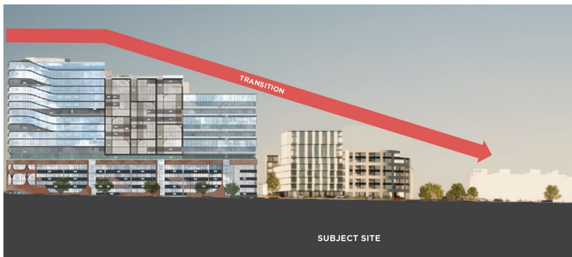
Figure 1 – Built form transition from north to south along Chandler Highway with a reduction in height of two levels to both Building A and Building B, and Level 8 deleted on Building D (Source: Elenberg Fraser with annotations)
