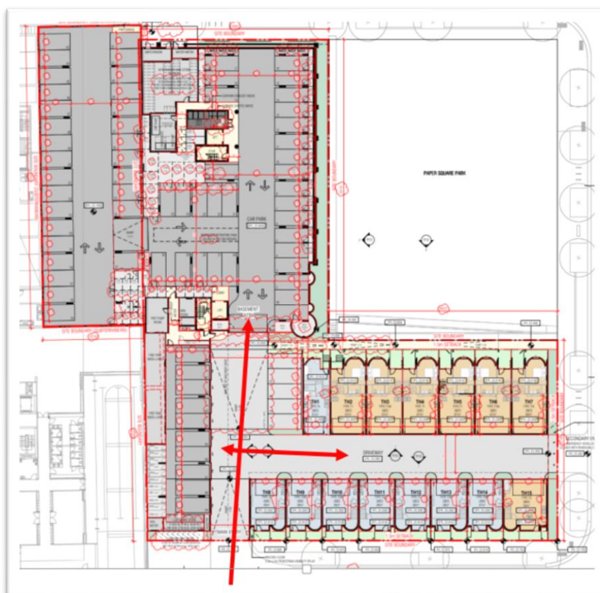
Figure 2: Vehicle and basement access
