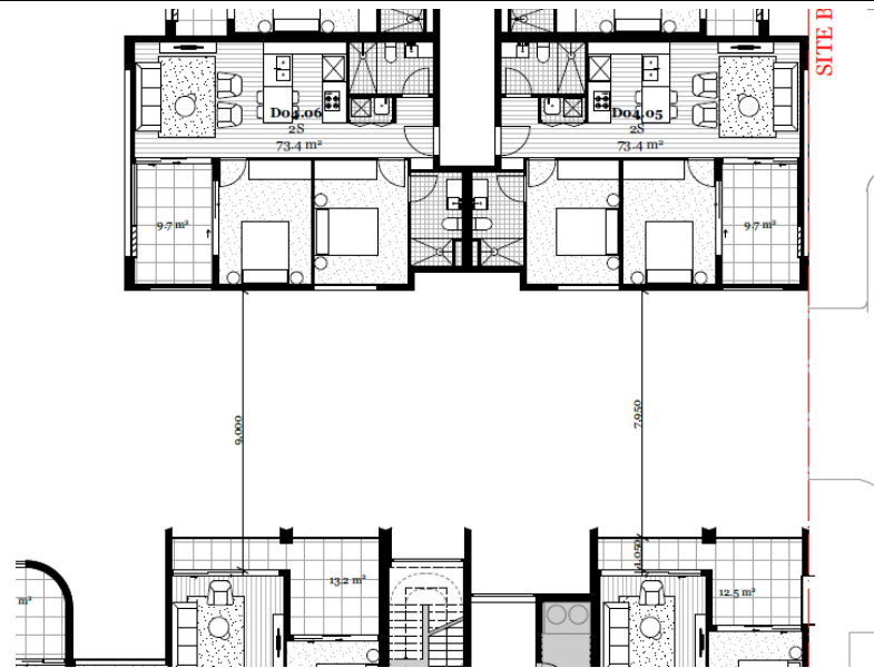
Figure 33 – Separation between Buildings C and D (Level 4)
