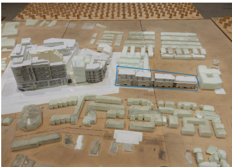
Figure 25 – 1:400 scale model for wind tunnel (Source: MEL Consulting report)
