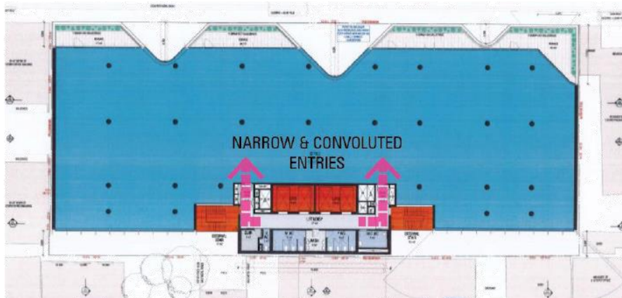
Extract of TP2003 Rev B showing recommend widening of smoke lobbies to visually enhance connection between office and core
