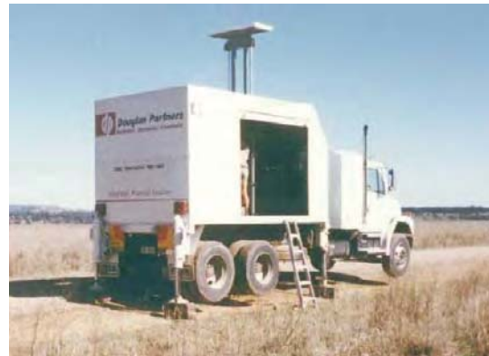
Figure 2: Purpose built CPT rig
