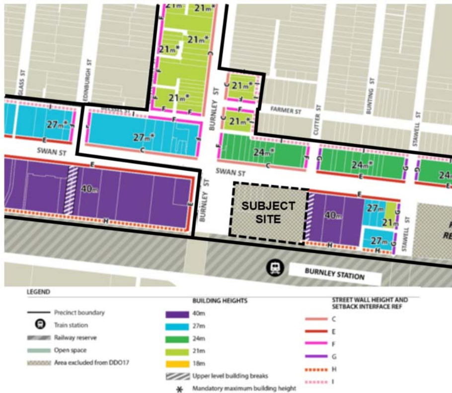
Note: All heights are preferred maximum building heights except where mandatory maximum building heights are shown Figure 15: Extract from Plan 5 (Precinct 3) and Plan 7 (Precinct 4) of proposed DDO17 (precinct boundaries shown as thick black line), detailing the proposed controls and location of the subject site.
