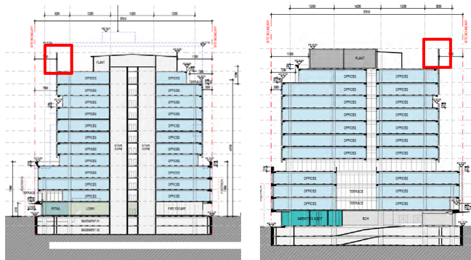
Figure 20: Section B-B and Section C-C showing the 6 metre high parapet proposed to conceal roof plant along the Swan Street interface
