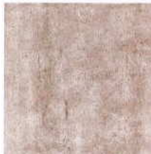
EF-18 STAINED PRE-CAST CONCRETE (TERRACOTTA COLOURED)
