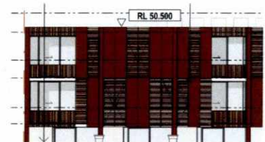
North oriented perimeter windows at level 3-4 of the west block are provided with horizontal slats.
