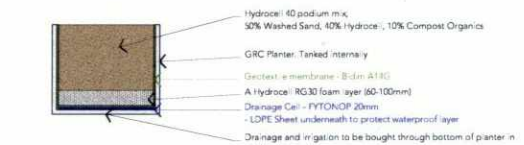
1 TYPICAL DETAIL - Planter Soil Profile 01-07 1:25
