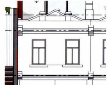
West oriented windows at ground floor and north and west oriented windows at level 1 are limited in size to reduce summer heat gains and winter heat loss.
