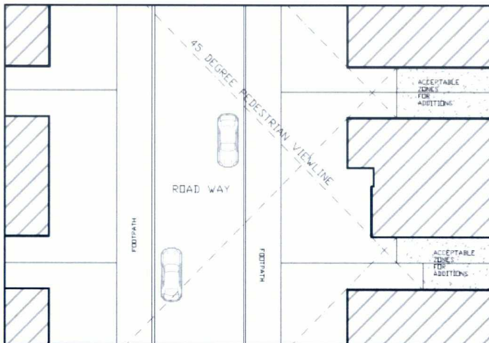
Figure 23 Diagram included at Clause 22.02 showing acceptable areas for ground level additions are sited within the area created by drawing a 45 degree view line from the opposite footpath through the front corner of the subject building and the corners of adjacent buildings Source: Clause 22.02, Yarra Planning Scheme
