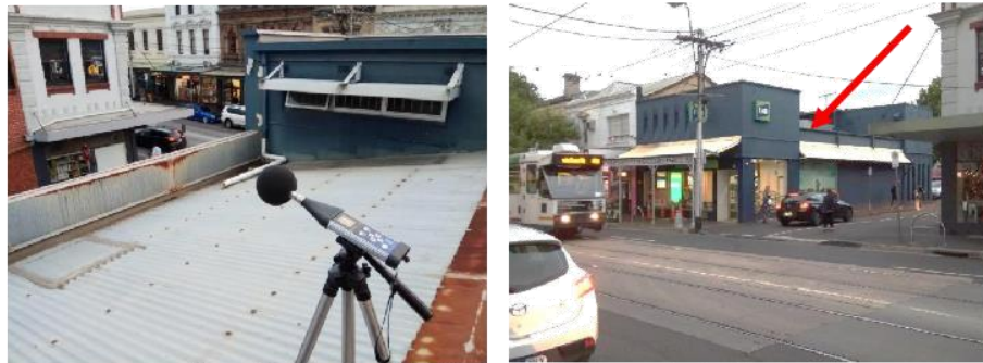
Figure 10 Location of the Sound Level Meter on the Roof
