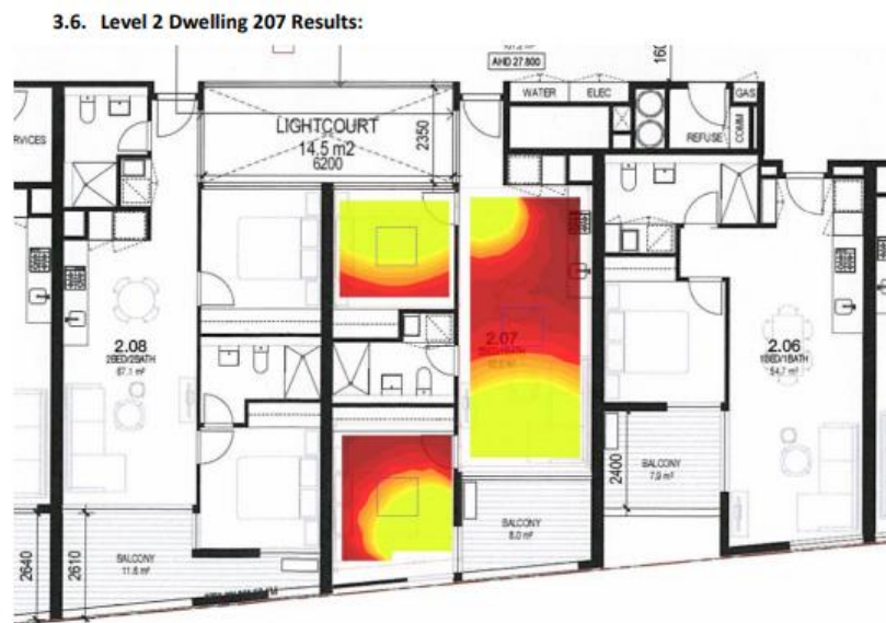
Figure 5 Dwelling 207 Bedrooms & Kitchen/living
