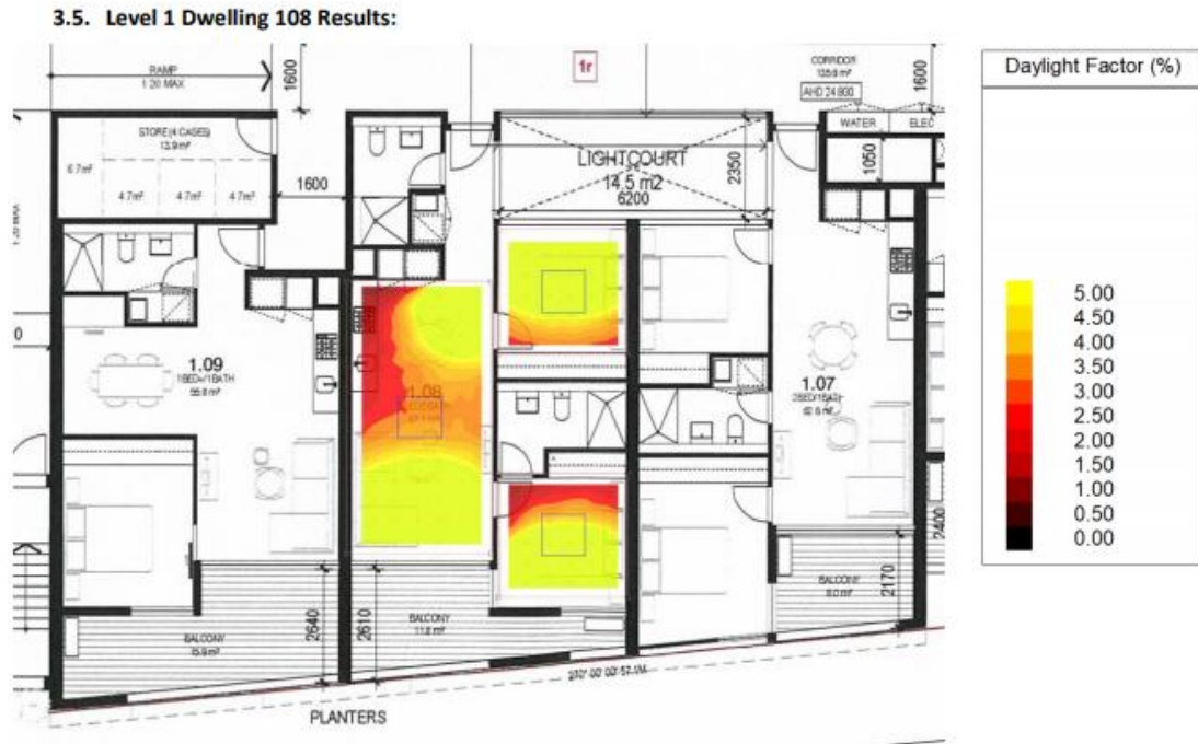
Figure 4 Dwelling 108 Bedrooms & Kitchen/living
