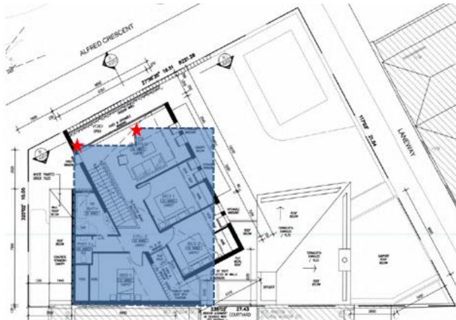
Figure 5: Existing building footprint overlaid on proposed new building showing existing setback points from Alfred Crescent (Heritage referral comments)
