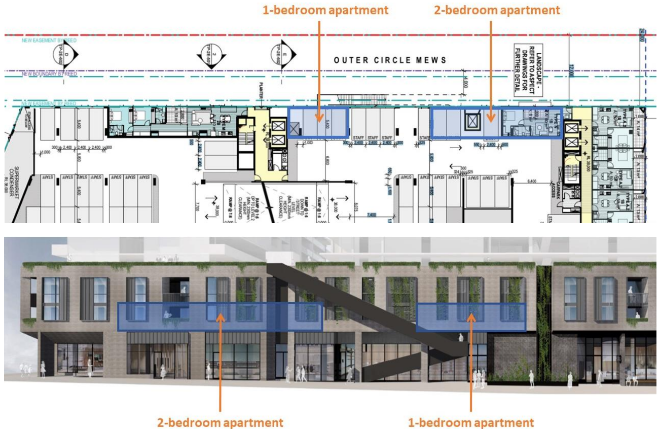
Extracts of Level 1 Plan and detailed Outer Circle Mews podium elevation showing potential location of additional apartments to activate the lane
