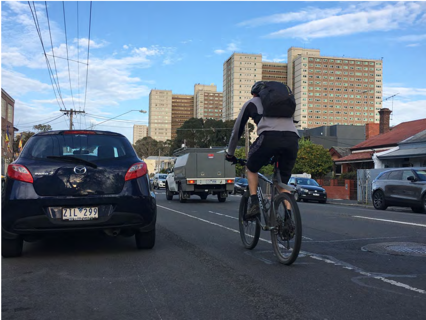
Elizabeth Street (Looking West): Narrow bike lanes place bike riders between the car dooring zone and moving traffic
