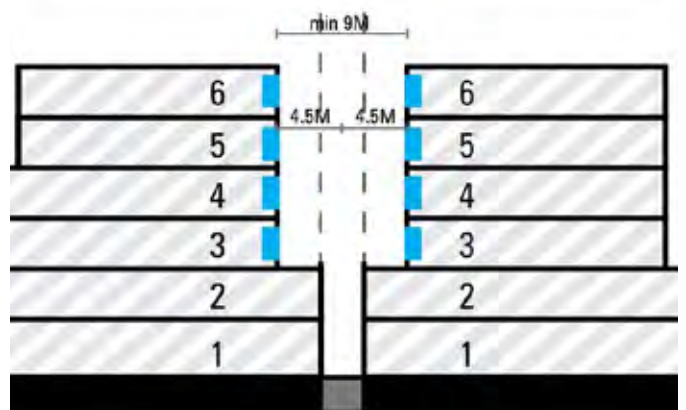
Cross-section of minimum 4.5m setback from habitable room window from centre of a laneway at upper levels
