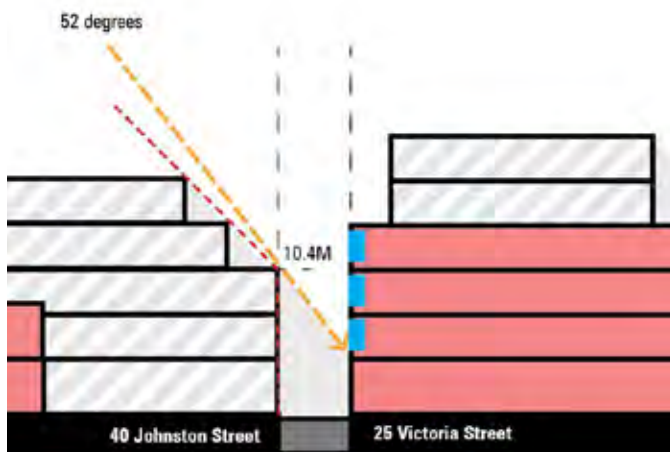
Cross-section of east-west laneway response to existing habitable room windows and balconies
