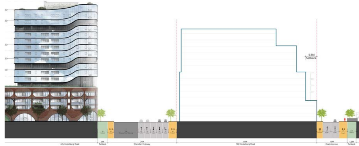
Figure 92. Alternate proposal supported by the applicant's expert witness for increasing the upper level setbacks on Coate Avenue to 5.5 metres
