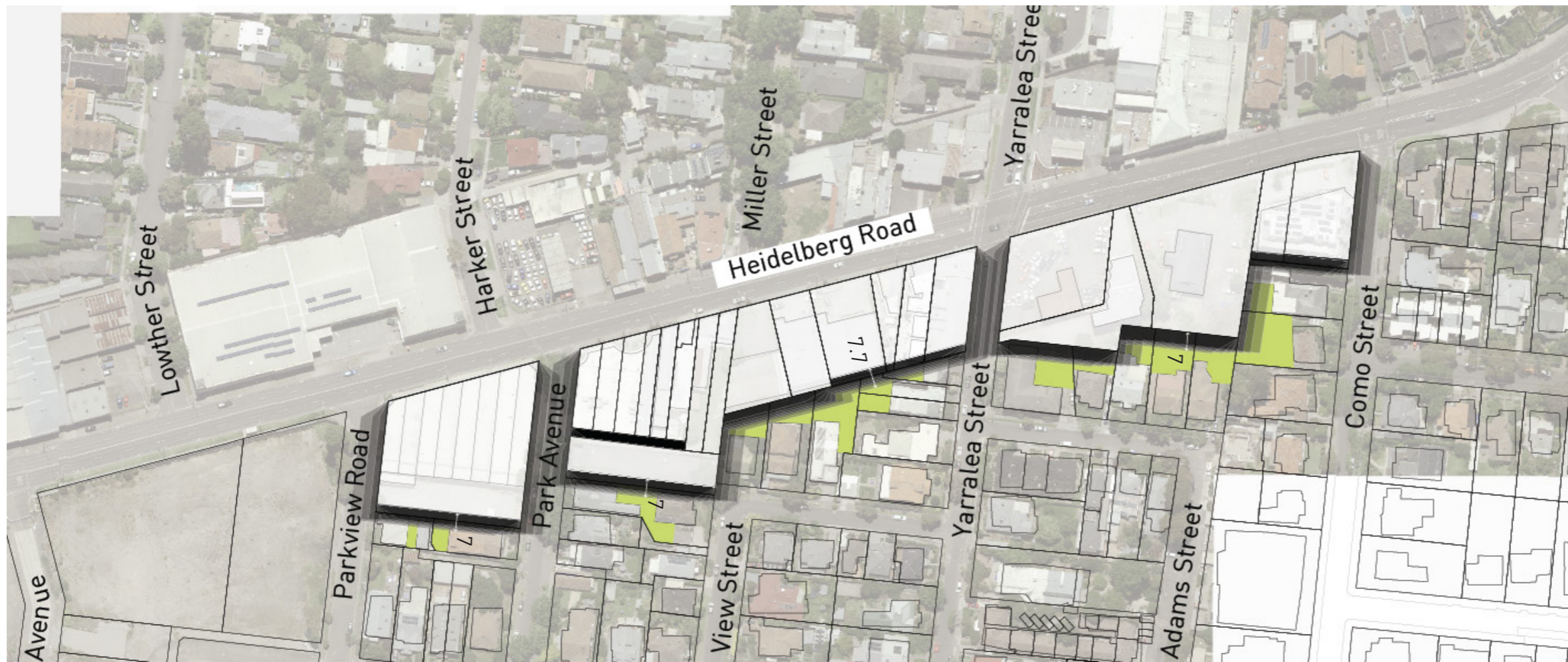
Figure 138. Cumulative shadow impact of 8 metre high boundary wall condition
