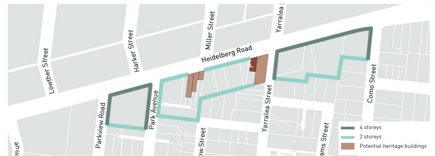
Figure 145. Precinct 3B - Proposed street wall heights / building heights along residential interface boundaries
