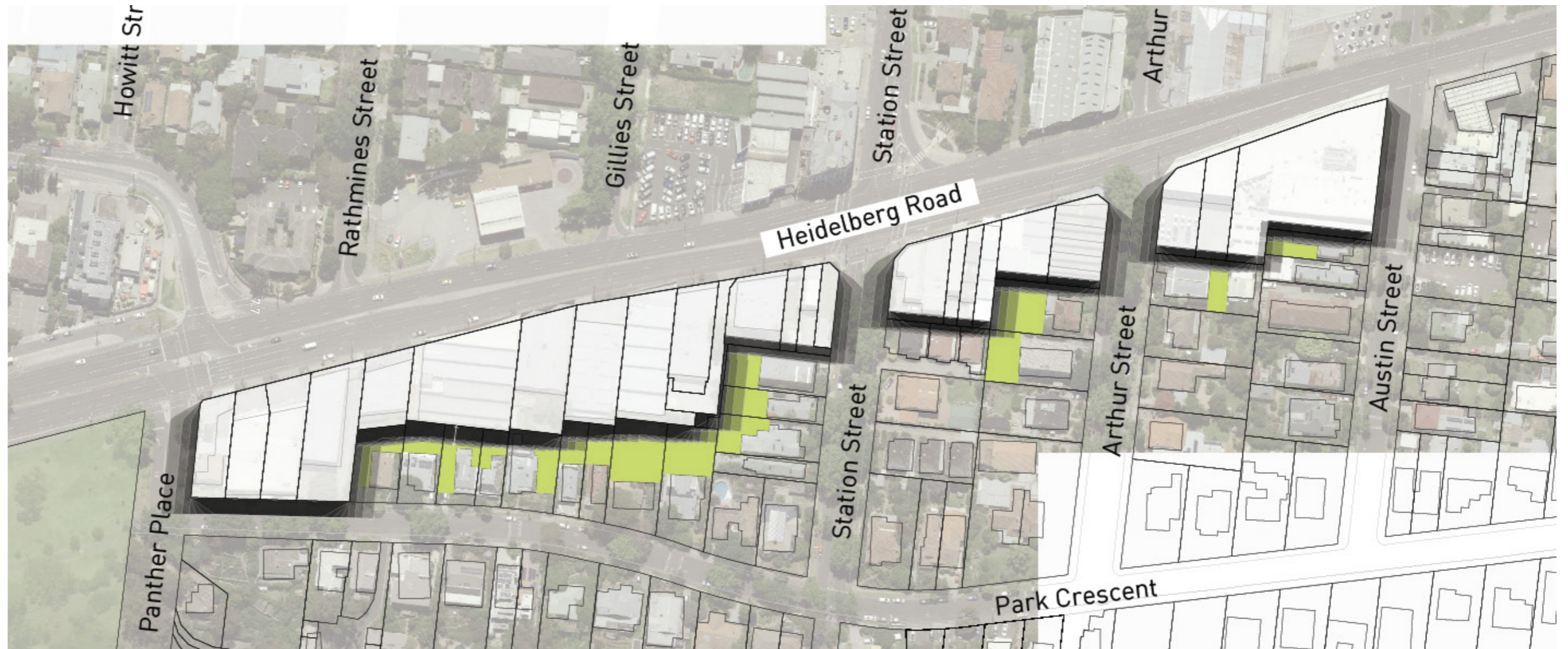
Figure 76. Cumulative shadow impact of 8 metre high boundary wall condition
