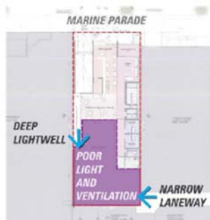
Poor light and ventilation to the Ground and Level 1
