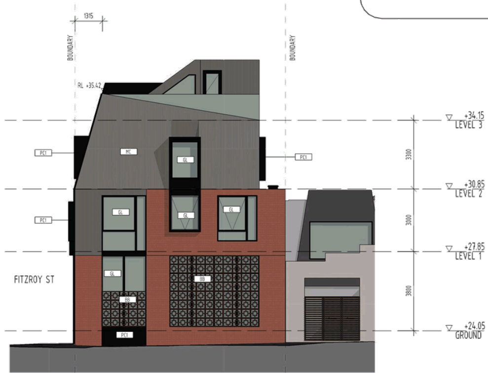
1 NORTH ELEVATION COLOURED 1 : 100
