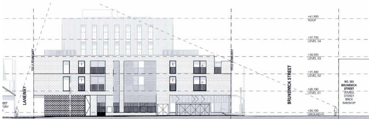
Above: Sightline diagram showing extent of visibility of rooftop development from directly across Brunswick Street.
