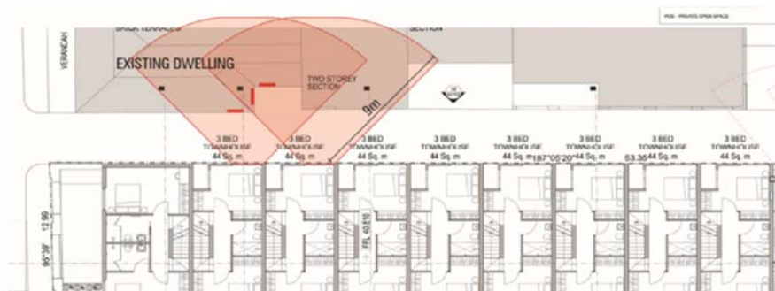
Existing windows of dwelling within 9m of the proposal (shown in red)
