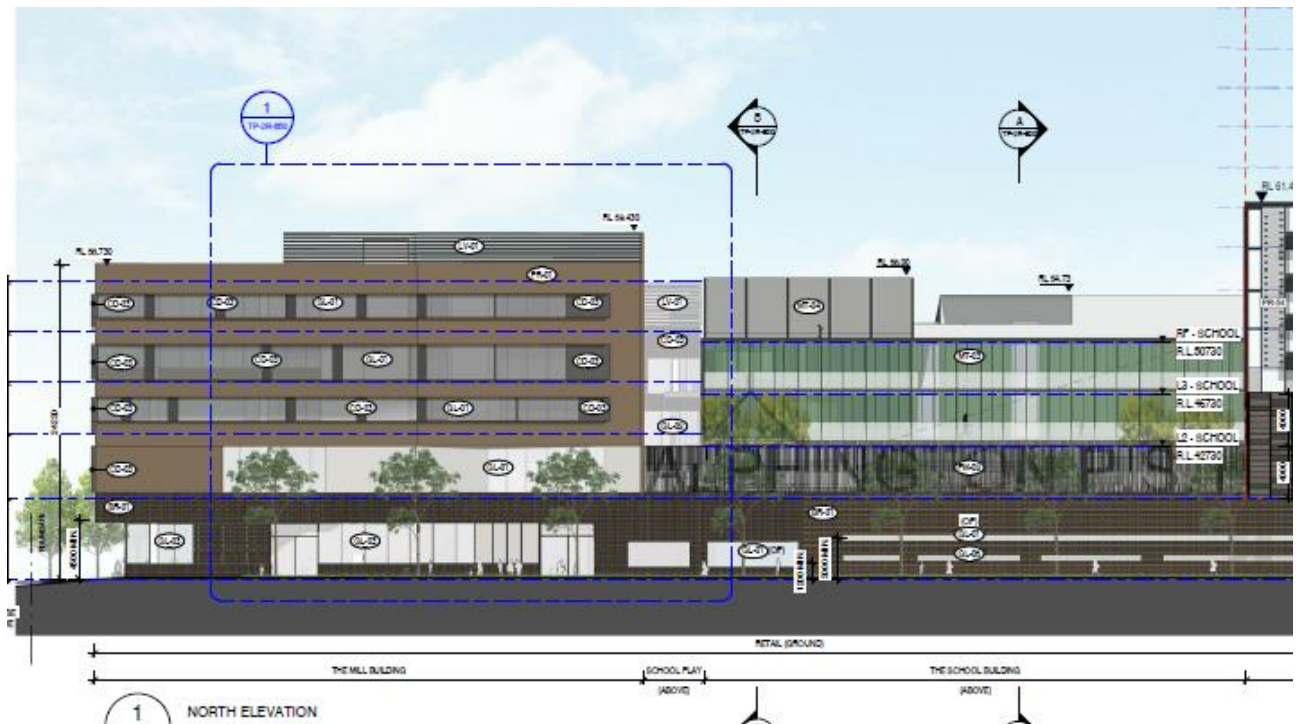
Figure 15: Part North Elevation – The Mill Building and abutting School.
