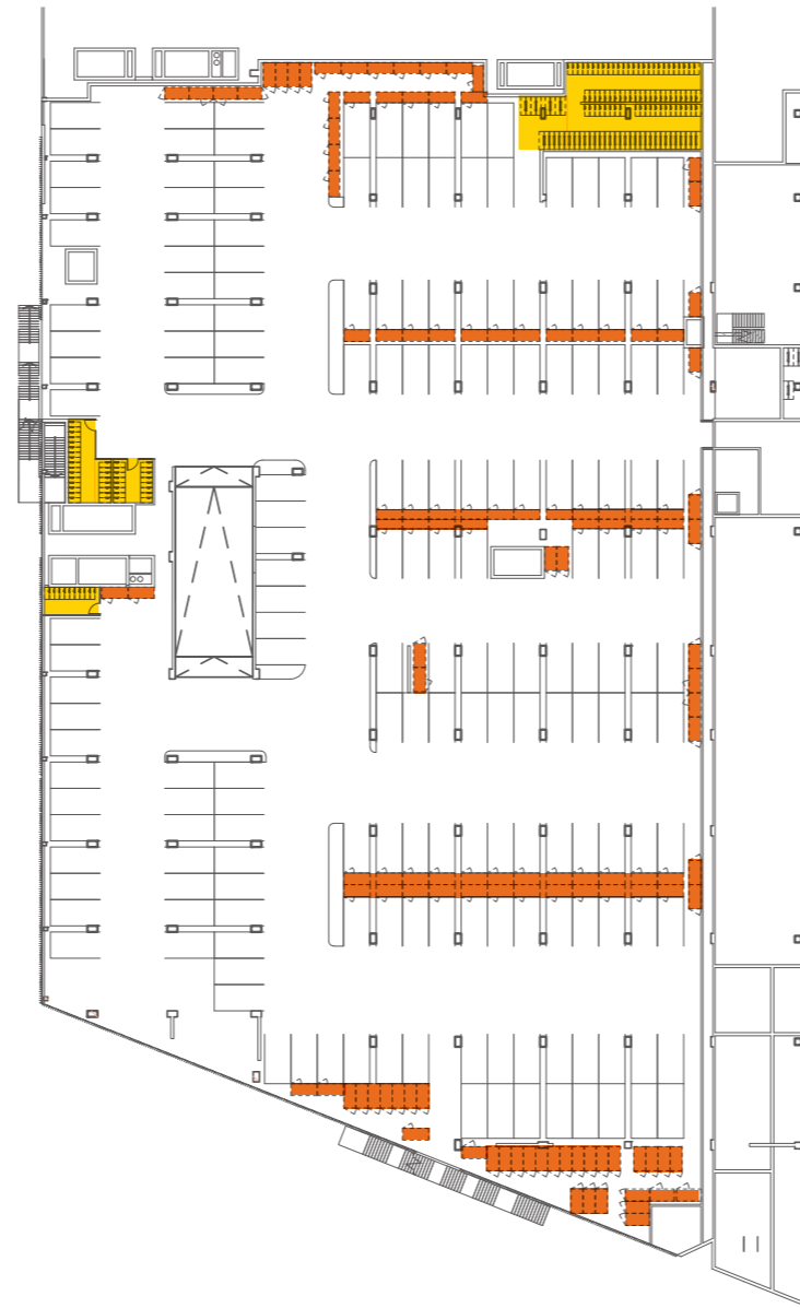
Figure 8.1.8.2 Level 1 Residential Storage and Bicycle Storage
