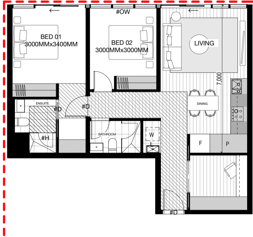
APT TYPE H 2 BED + STUDY INTERNAL STORAGE: 9m3 min. 85sqm URBAN ANCHOR - Lvl 03-13
