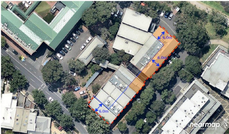
Figure 23. Minimum acceptable setbacks, roof retention and façade retention (including the 1984 link structure and projecting elements on Yarra River elevation of the 1920s factory building)
