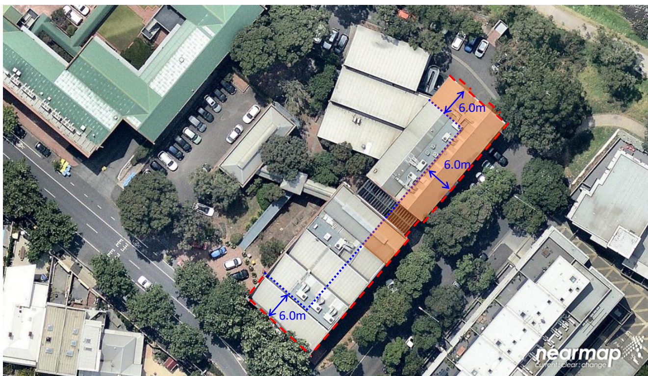
Figure 9. Figure 23 from Mr Gard’ner’s evidence showing minimum acceptable setbacks, roof retention and façade retention (including the 1984 link structure and projecting elements on Yarra River elevation of the 1920s factory building)
