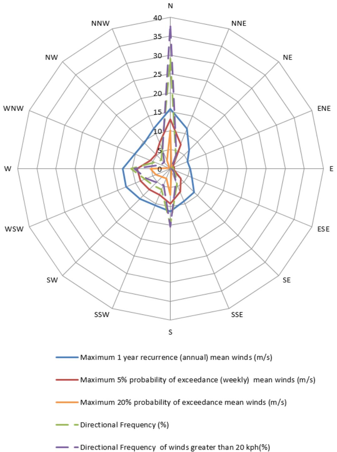
**Figure 2: Annual, Weekly Recurrence and 20% (probability of exceedance) Mean Wind Speeds, and Frequencies of Occurrence, for the Melbourne Region (based on 10-minute mean observations from Melbourne Airport from 1970 to 2009, corrected to open terrain at 10m)**
