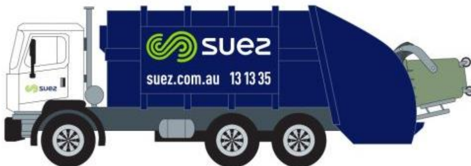
Figure 5: Typical SRV rear-lift waste collection vehicle
