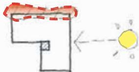
Linear type form - building width oriented to north. West & east facades suffer from low angle sun. Requires extensive external shading to avoid overheating and glare.
