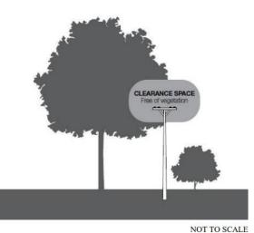
FIGURE 5 – UNINSULATED 66 000 VOLTAGE ELECTRICAL LINE IN A LOW BUSHFIRE RISK AREA Clauses 27, 28 and 29, Graphs 4, 5 and 6
