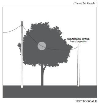
FIGURE 3 – INSULATED ELECTRICAL LINES IN ALL AREAS AND UNINSULATED HIGH VOLTAGE ELECTRICAL LINES (OTHER THAN 66 000 VOLTAGE ELECTRIC LINES) IN LOW BUSHFIRE RISK AREAS
