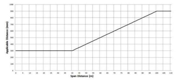
Appendix 3 – Applicable distance for middle two thirds of a span of an electric line GRAPH 1—INSULATED ELECTRIC LINES IN ALL AREAS
