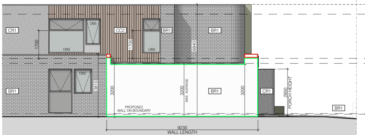
Figure 9: Proposed wall on boundary with compliant area (green) and area exceeding 3.6m (red)
